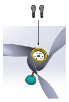
Remove 3 screws from LED fixing plate (1), place the light housing on it, and tighten with the same 3 screws (2).
