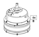
Place the motor assembly as shown and remove all 6 blade screws (A) from bottom side of motor. Turn the motor around and open 6 blade screws (B) from top side also.
