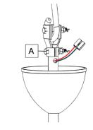
Tighten with washer, nut, lock nut and cotter pin in sequence as written.
