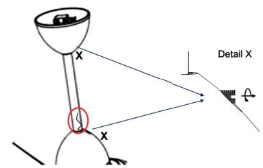
With screws (X) tightened, there can be scratches incurred on down rod on movement of canopy.
