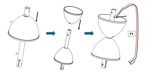
Insert bottom canopy (2) from top end of down rod (3) (no-slit end). Insert top canopy also from same end.
