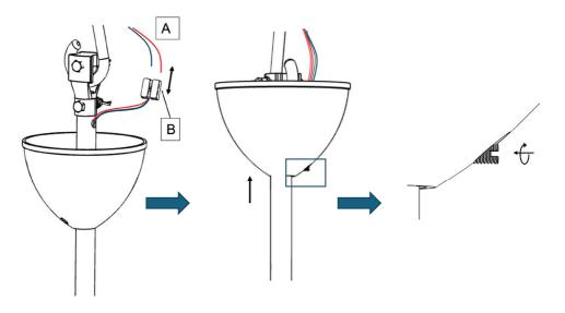
Connect the wires from main supply (A) into fan connector (B).
