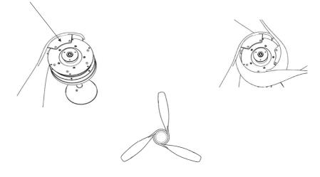
Screw 6 blade screw on bottom plate. Place the motor with light side up, and install all blades with blade screws on top and bottom plate.
