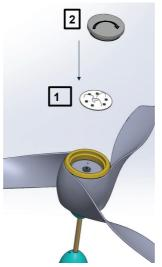
Fasten the LED (1), make wire connections , and close with diffuser (2).
