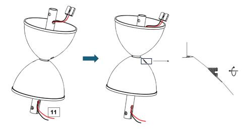
Take the supply wire (11) out from the slit-end of down rod. (3)
