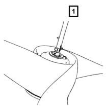
Remove 3 screws from false cover fing bracket (1), place the false cover on it, and tighten with the same 3 screws (2).
