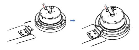
Bring the 1st Blade towards the fan motor, and align with the blade holes on the motor unit
