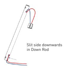
Take the DownRod with pre-inserted supply wire
