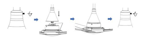
Loosen he Screw and Brin he lower Canopy down Fasten back the Screw lock the canopy in position
