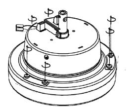
Place the Motor unit over a towel on a table, and open the 6 Blades and Screws as shown
