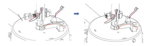
Fasten the Down Rod bolt as shown
