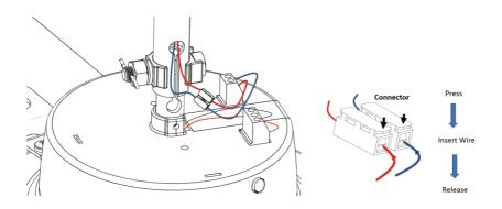
Connect the Supply wire from Down Rod into Link Wire connect Wire Connection Method
