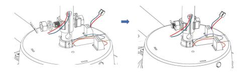
Insert Down Rod slit-end down over Motor Shaft
