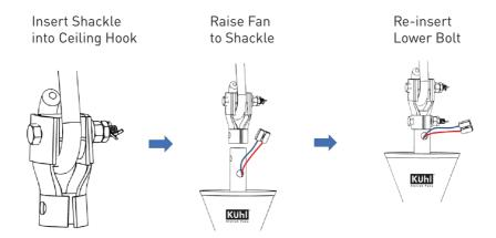
Tighten with Washer, Nut, Lock Nut and Cotter Pin in sequence as written
