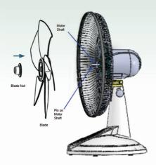
Take care of the slots in blade hub inserted onto the pin on the motor shaft. Finally re-tighten the blade nut turning it anti-clockwise.
