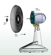
There are 3 pins on motor and 3 holes on guard. The holes have to be inserted into the pins. Thereafter tighten with guard nut.
