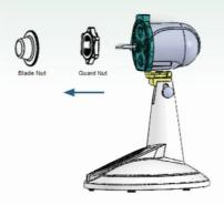
Blade nut has to be unscrewed turning clockwise and rear guard nut by turning it anti-clockwise.
