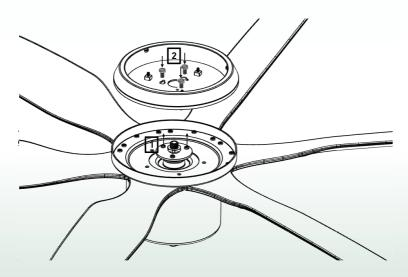
Remove 3 screws from LED Fixing Plate (1), Place the Light Housing on it, and tighten with the same 3 screws (2)
