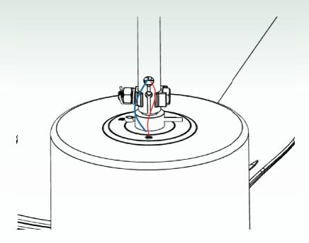
Make Input Electric connection into the Connector coming out of Fan
