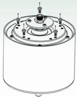
As shown in the figure, remove all 5 motor screws
