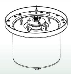
Assemble the Blade Housing with previously removed screws
