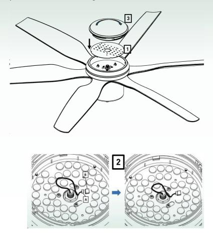
Fasten the LED (1), make wire connections (2), and close with diffuser (3)
