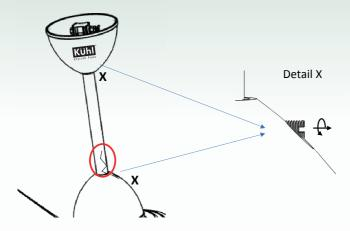
With screws  ${\bf X}$  tightened, there can be scratches incurred on Down Rod on movement of canopy.
