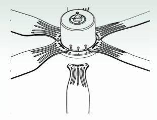
Turn the fan over and install blades with blade screws provided on Blade Housing
