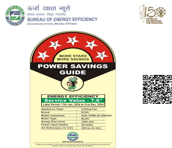
The unique label series code provided in the letter has to be mentioned in the label affixed on the Electric Ceiling Type fan.
